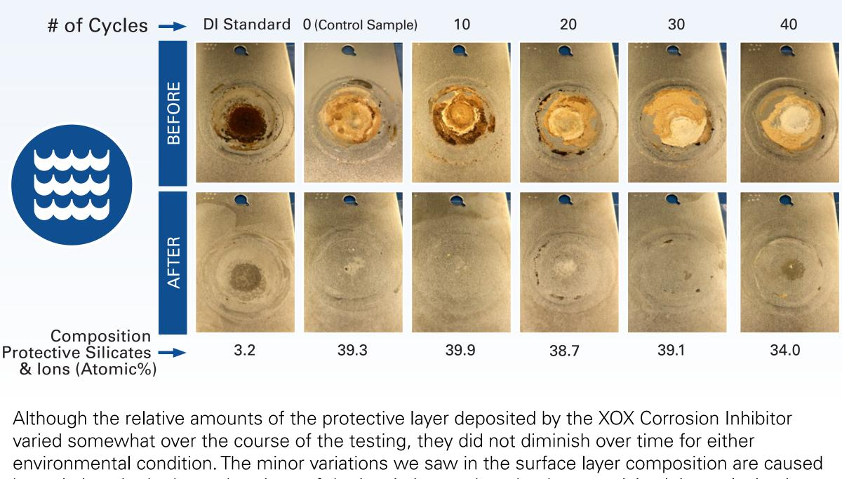
by variations in the base chemistry of the insulation, and not by the material gaining or losing its corrosion inhibiting properties as a result of wet-dry cycling.
